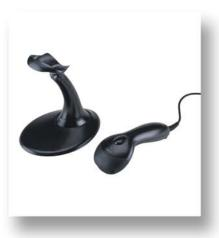
menu-scanning. When the MS9540 is placed in its stand, CodeGate can be automatically deactivated allowing **Voyager**cs to be used as a fully automatic presentation scanner.
